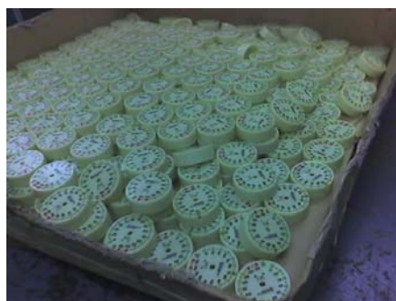
Sherwood SPG Faces Used in assembly of SPGs at Oceanic Each SPG is individually calibrated
