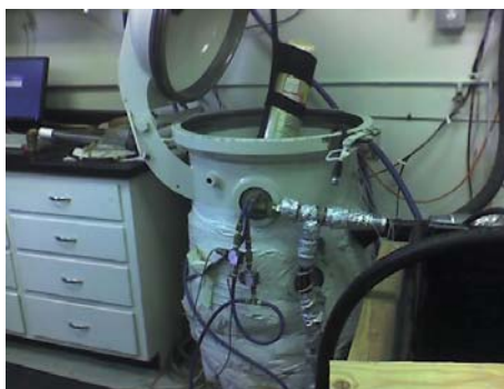
This little pressure cooker allows Oceanic to perform quick pressure checks on regulators at depth, as part of its work with Scuba Lab
